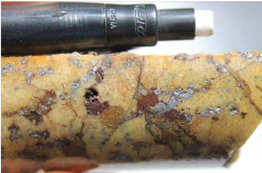
*Photograph; Massive quartz vein with chalcopyrite and molybdenum rosettes at 164.00m (photo from Menzies and Corbett 2015), from 6 metre interval which reported 2.64% Cu and 908 ppm Mo from 158 metres downhole (see GBM ASX Report for the Quarter Ended 31<sup>st</sup> December 2014).*
