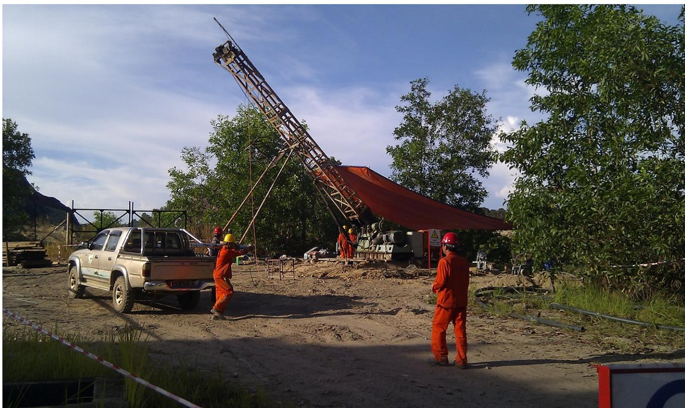
Photograph; Drilling of hole LMD011 testing the Western Shear Zone. The Lubuk Mandi Main pit is behind the rig (obscured by vegetation).
