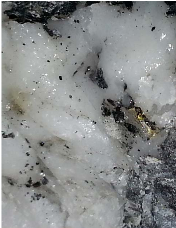
Photograph; Fine native gold particles in vein quartz from MSZ in LBD010. Field of view approximately 1 centimeter.
