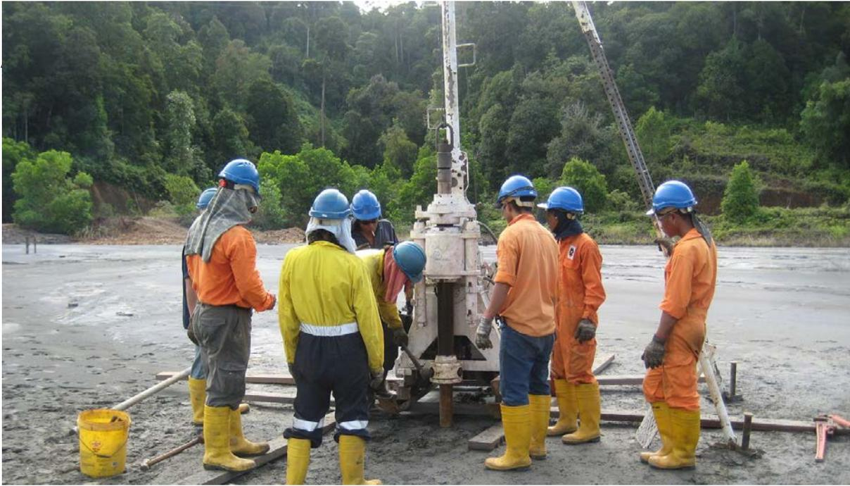
*Drilling of tailings target on Lubuk Mandi. Drilling utilized standard diamond drilling equipment with a finger lifter to retain wet tailings samples.*
