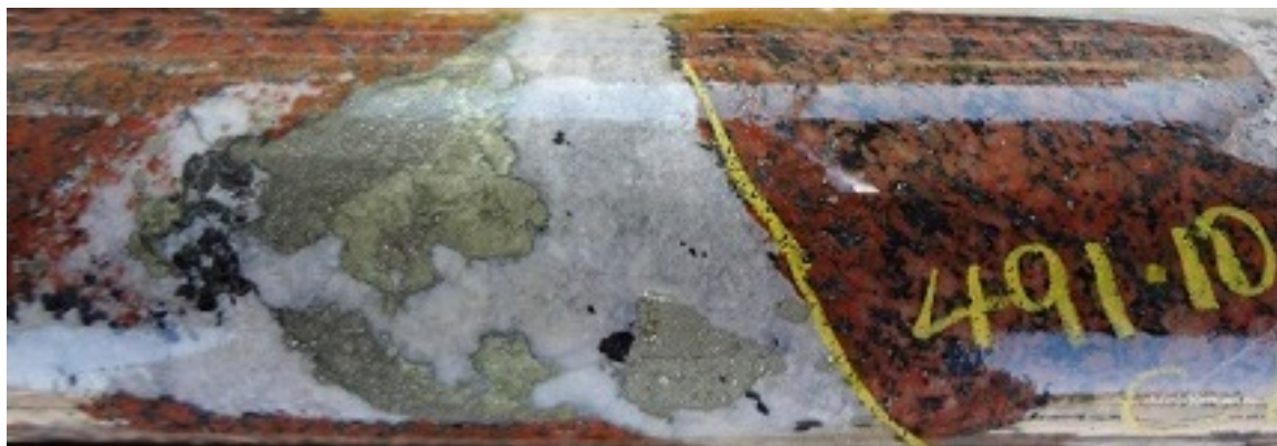
Photograph: Chalcopyrite + pyrite in a carbonate + chlorite + magnetite vein at 491.1m down drillhole BNG003 at the Bronzewing Bore prospect.
