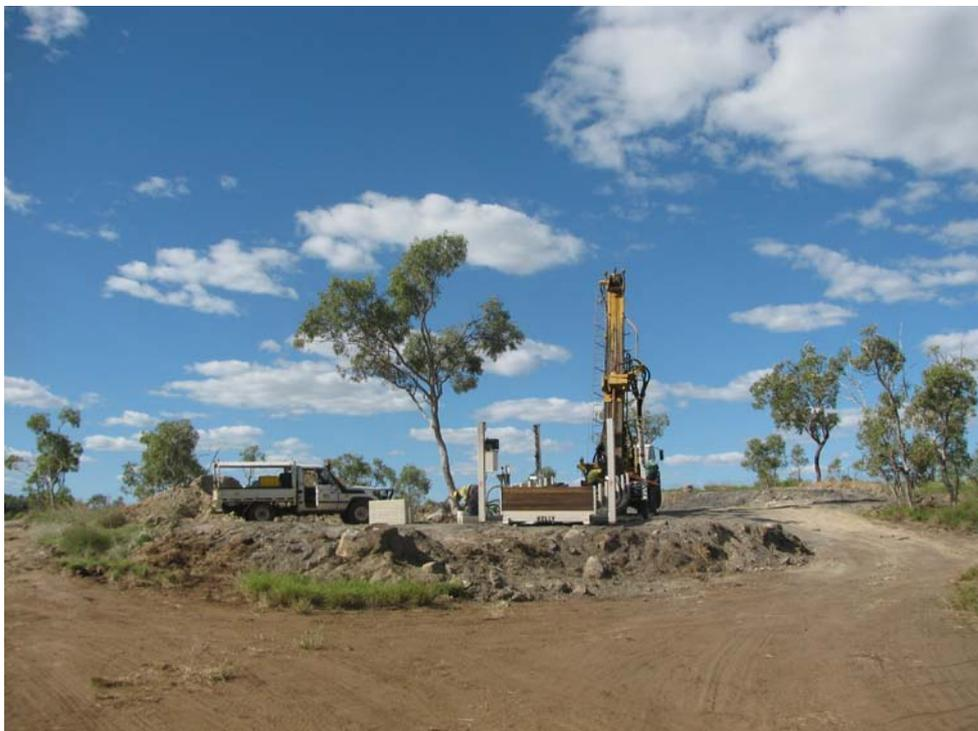
*Picture: Diamond drilling at the Milo Prospect.*
