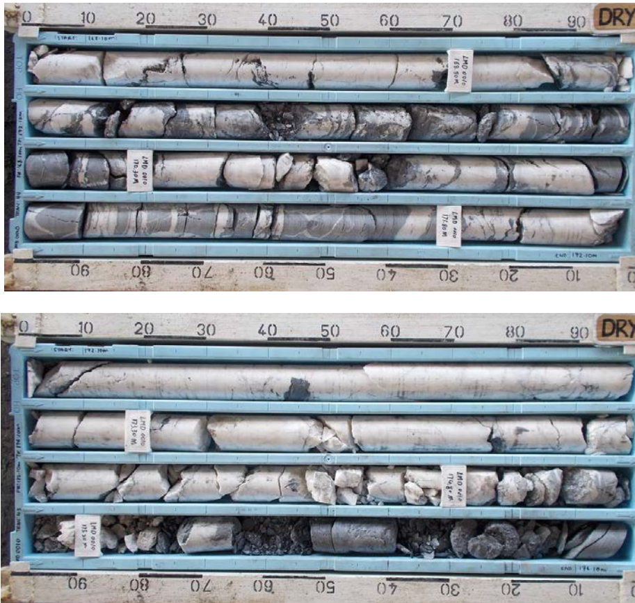
Photographs; HQ Drillcore from MSZ intersection in LMD010 showing extensive quartz veining and shearing.
