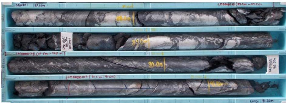
Photo of representative diamond drill core from drillhole LMD0001 at Lubuk Mandi showing intense shear fabric, quartz breccia and stockwork intersected within the target Eastern Shear Zone.
