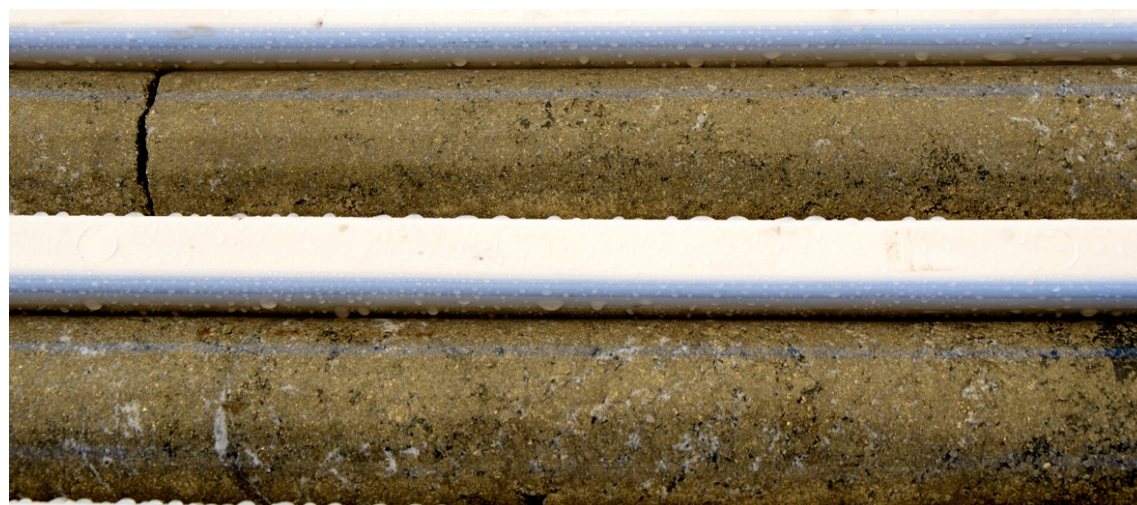
Photograph 1: massive sulphides (largely pyrite) in wet drill core from 132 metres in drill hole MD014 (NQ2 drill core, diameter 53mm).
